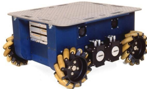
Uranus, CMU: Omnidirectional Drive with 4 Wheels
