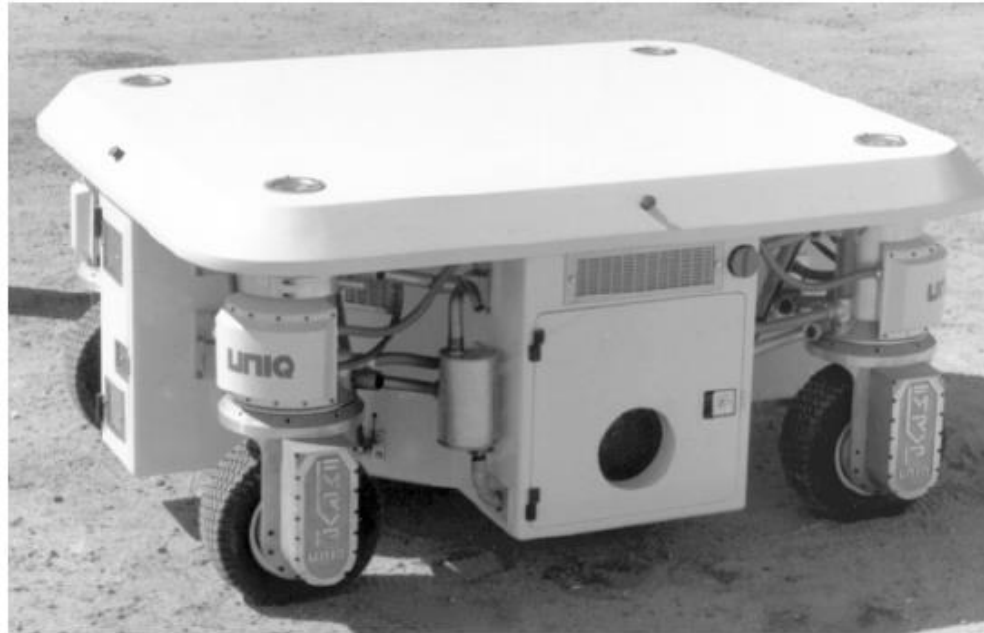
An 8-DOF platform with four wheels individually driven and steered.
