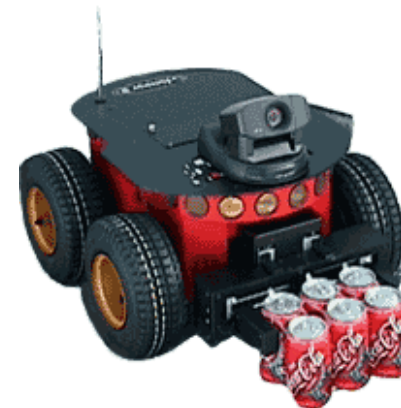
Non-holonomic Robot Robot can move in some directions (forwards and backwards), but not others (side to side).
